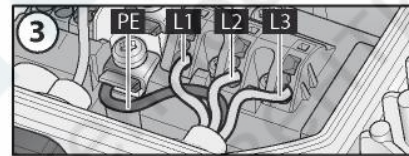
Fig. 2: Connecting wires to terminals
